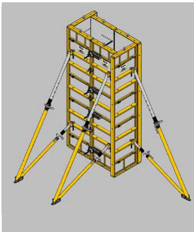
▲ Dwarf wall joined with clamps and LGR waler.
